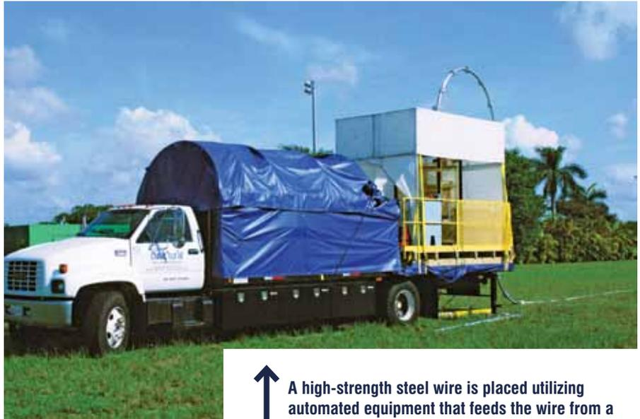
↑ A high-strength steel wire is placed utilizing automated equipment that feeds the wire from a truck unit positioned outside the access way.
